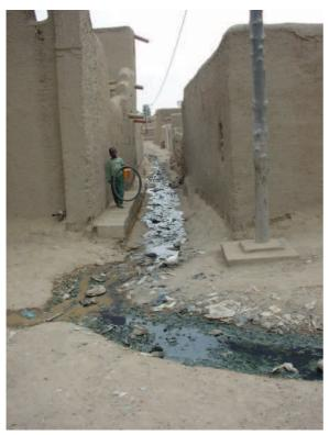
Figure 8 - Accumulation and stagnation of wastewater on the street
